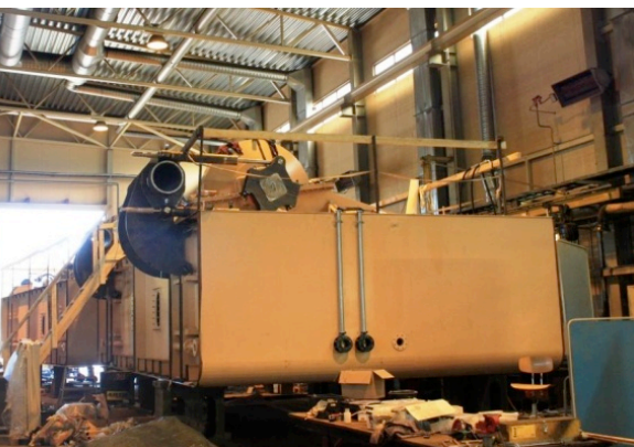
300 kW WaveRoller – Machine room Source: AW-Energy
