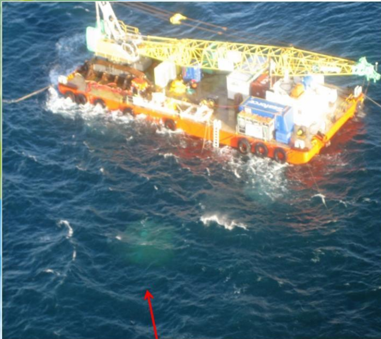
Fully submerged Commercial Scale CETO unit in operation next to deployment barge
